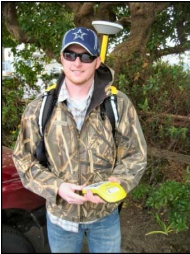
Geology Honors student Michael Snyder equipped for the field with our Trimble handheld GPS unit with attached backpack and 'Hurricane' antenna for better accuracy.
