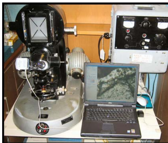
Petrographic microscope with attached laptop computer and digital camera.
